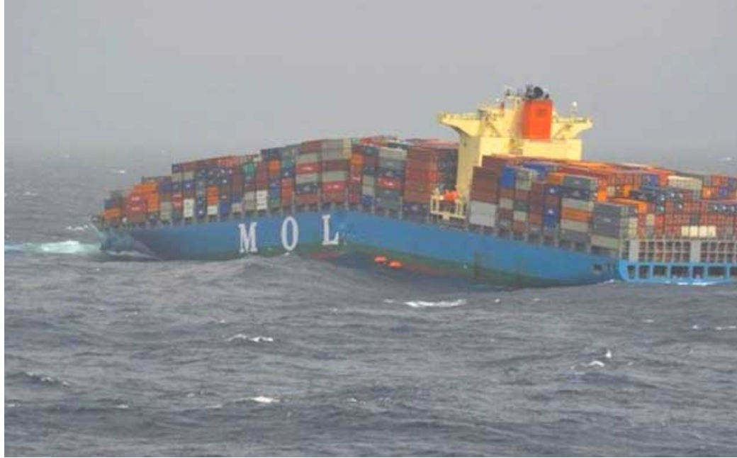
Figure 1.1: MOL COMFORT after structural failure and before sinking
