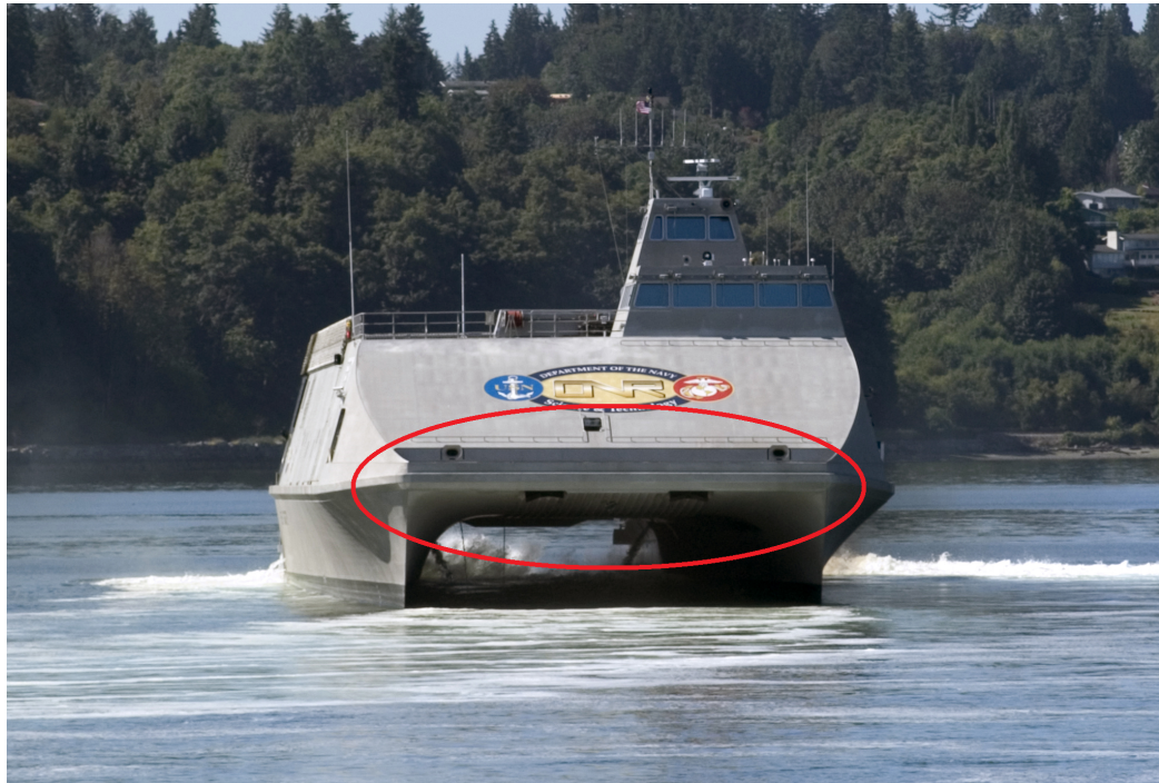
Figure 1.3: X-craft naval catamaran showing the design of a flat wetdeck circled in red
