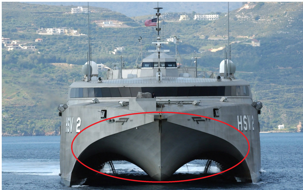
Figure 1.4: The naval HSV-2 Swift catamaran with wave piercing bows and a wedge shaped wetdeck to mitigate slamming loads
