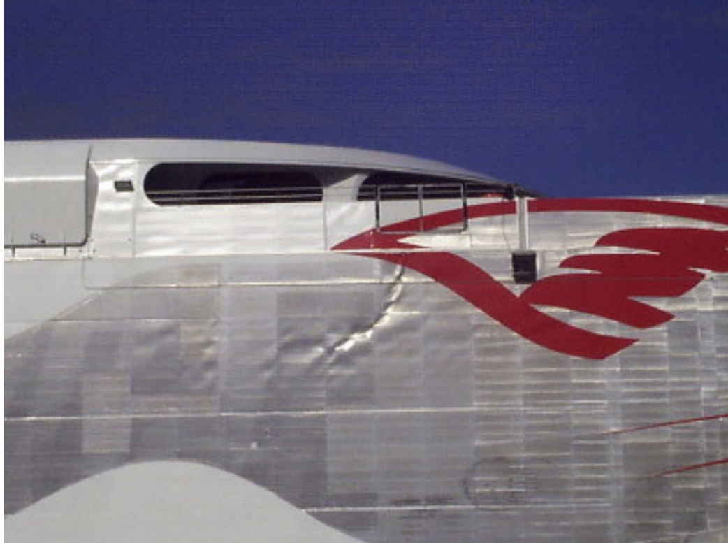
Figure 1.2: External plate buckling after an extreme slam event Lavroff et al. (2013)
