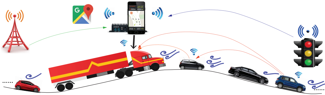
Figure 1.6: Traffic level: safe and fuel efficient connected cruise control strategy that also responds to elevation.
