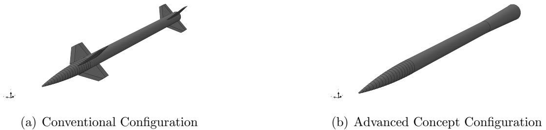
Figure 3.3: Vehicle model outer mold lines for the state of the art and concept configurations being considered.
