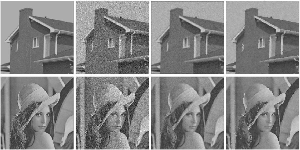
Figure A2: Restoration of images. For each row, from left to right: original image, image with Gaussian noise added, image restored using Gaussian smoothing with a 5 \times 5 kernel and image restored using proposed algorithm.
