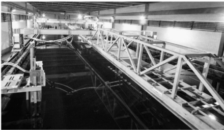
(a) Suspended guide ditching system
