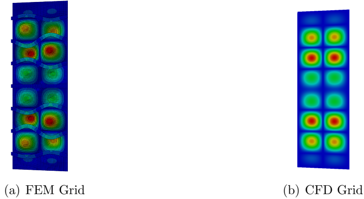
Figure 6.3: Illustration of mapping between the fluid (a) and the structure (b)
