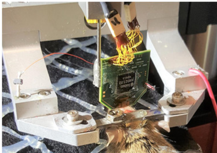
Figure 4-13. In vivo measurement setup of the headstage. The optoelectrode is implanted into an anesthetized mouse.
