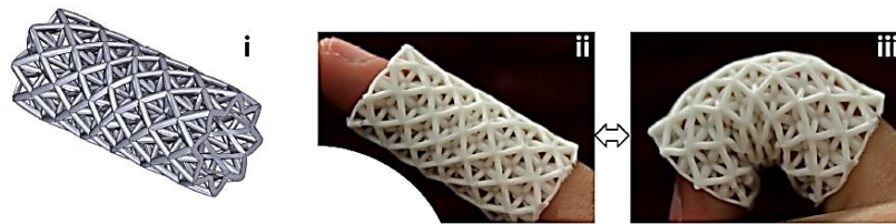
Figure A-44. Elastomer metamaterials (Jiang & Wang, 2016).
