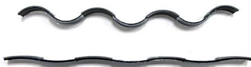
Figure A-8. An illustration of 1D-to-2D sinusoidal shape-shifting by self-bending (Tibbits et al., 2014).
