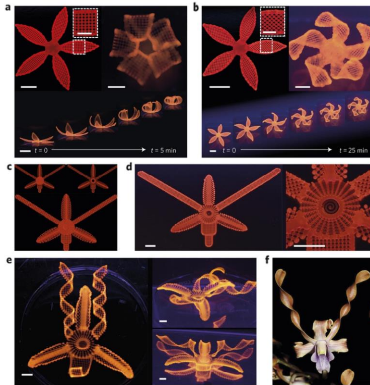
Figure A-33. 2D-to-3D shape-shifting by the combination of bending and twisting with complex flower morphologies (Gladman et al., 2016).
