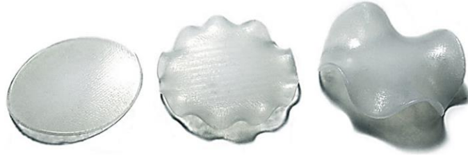
Figure A-32. 2D-to-3D shape-shifting with surface topography (Tibbits et al., 2014).
