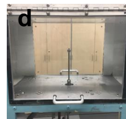
Figure 4-17. (a) Wind tunnel test on the samples installed on the sting, (b) flat sample attached to the sting, (c) deformed sample connected to the sting and (d) wind tunnel test on the pure sting.
