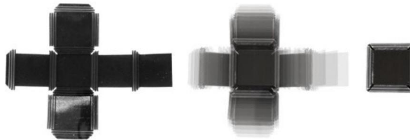
Figure A-22. An illustration of 2D to 3D shape-shifting by self-folding to make a cube (Tibbits, 2014).
