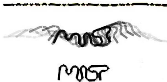
Figure A-7. The illustration of 1D-to-2D shape-shifting by self-folding (Tibbits, 2014).
