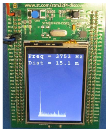
Figure 4.15. Microcontroller display showing beat frequency, range and FFT spectrum
