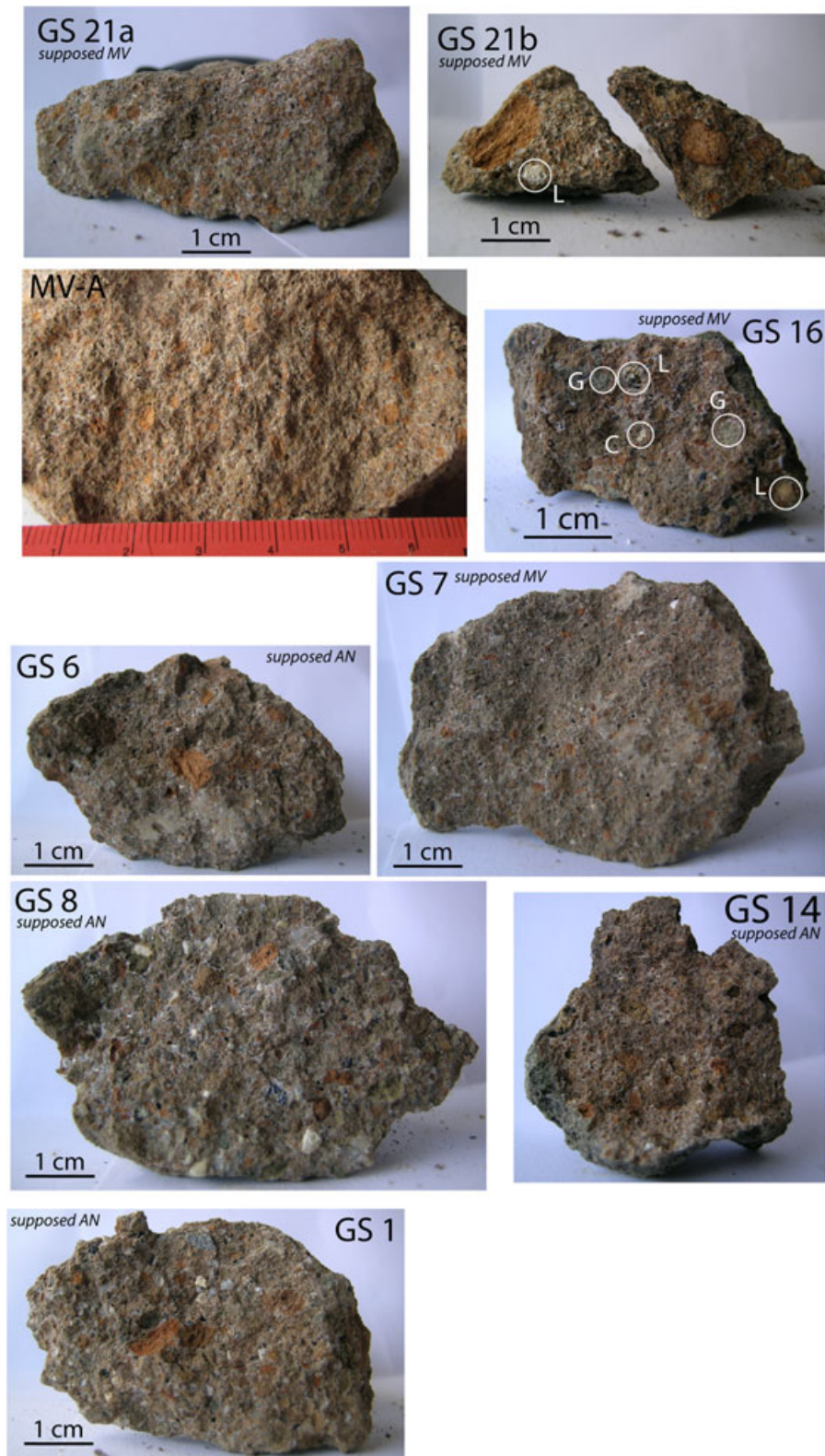
FIGURE 4 Photographs of tuff samples showing varying macroscopic aspect, from a rock facies (MV) similar to that of the Tufo Lionato cropping out in Monteverde (sample MV-A), to that typical of the Tufo Lionato cropping out in the AN. AN: Anio river valley; C: carbonate lithic clast; G: gray scoria; L: leucite crystal; MV-A: Monteverde facies
