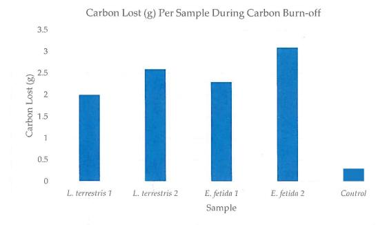
**Figure 5.)** Four terrariums of two worm species (*Lumbricus terrestris* and *Eisenia fetida*) were allowed to circulate compost into sandy soil for 12 days before the sand was homogenized and dried. Samples of the dried sand from each terrarium and a control were taken and placed into a muffle furnace at 500° C to burn off the carbon they contained. The masses of the samples were taken before and after carbon burn-off and the differences between those values are graphed above.
