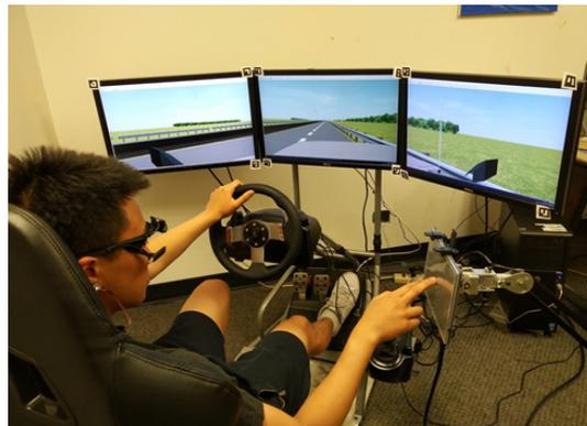
**Figure 3** Driving simulator and secondary task setup. This setup increased the realism of the experimental tasks. Markers were placed on each monitor and the touchscreen to identify surfaces for eye-tracking
