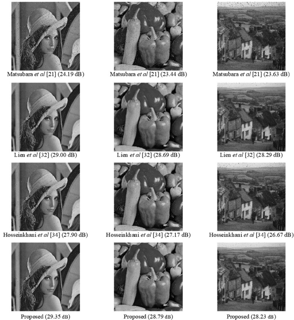
FIGURE 16 Visual quality comparison of the proposed method with Matsubara et al., 21 Lien et al., 32 and Hosseinkhani et al. 34 Peak signal-to-noise ratio (dB) values are also shown
