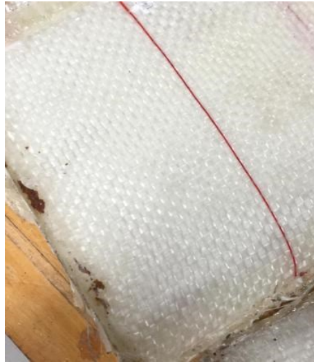
Figure 13. Sheild Strand S ® / Epoxy composite.
