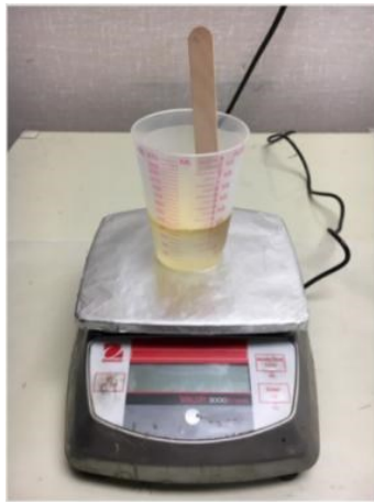
Figure 9. Epoxy resin mixture on a Digital weighing scale.
