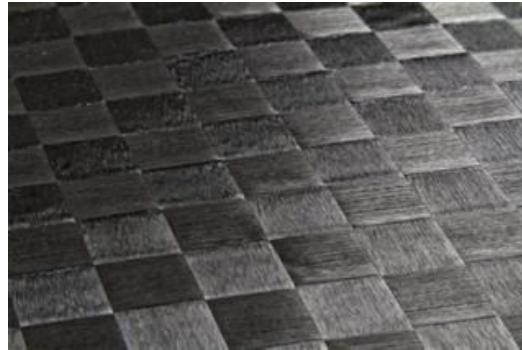
Figure 5. Spread tow fabrics for ultralight composites [19].
