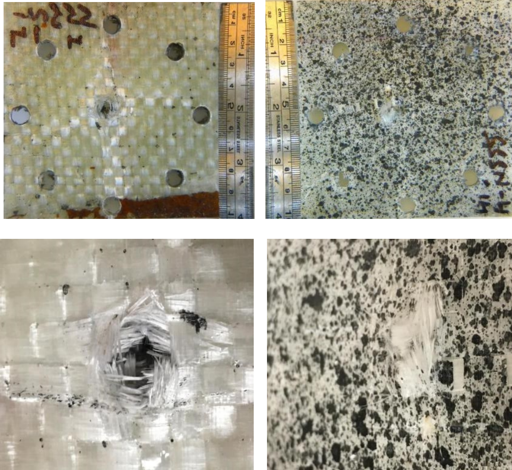
Figure 146. Shield Strand S® / Epoxy based 4.5 mm thick composite impacted at a velocity of 152.4 m/s with the sharp nose projectile.
