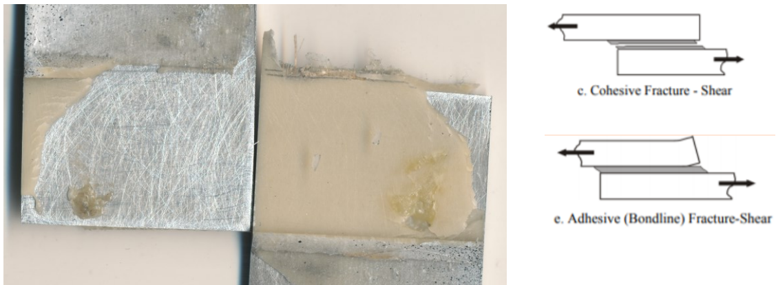
Figure 3.7 Low magnification image after fracture of Al-Al bonded with high strength epoxy under tensile loading conditions at a strain rate of 0.15 \text{ s}^{-1}
