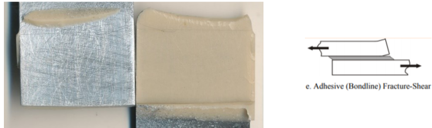
Figure 3.90 Low magnification image after failure for Al-CFRP SLJ bonded with high strength epoxy tested subjected to a strain rate of 150 \text{ s}^{-1} .
