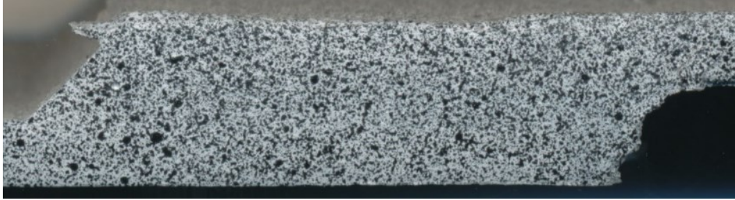
Figure 2.11 Typical speckle pattern required for DIC measurement.
