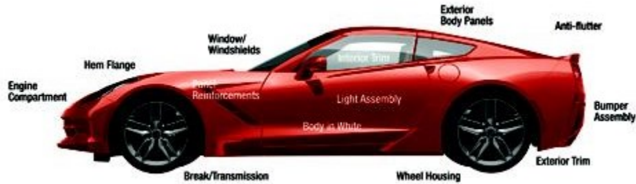
Figure 1.11 Body parts where adhesives are used in the automotive industry.
