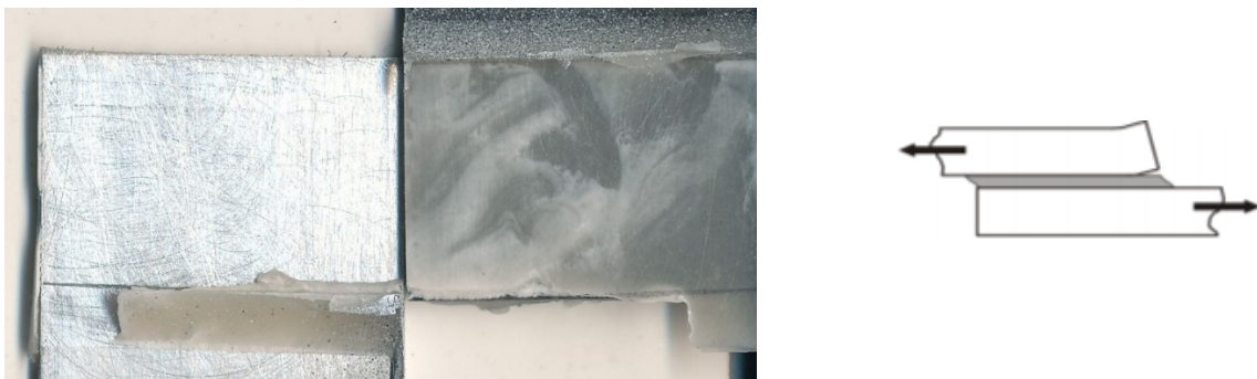
Figure 3.38 Low magnification image after fracture of Al-CFRP bonded with urethane-based adhesive at a strain rate of 0.0015 \text{ s}^{-1}
