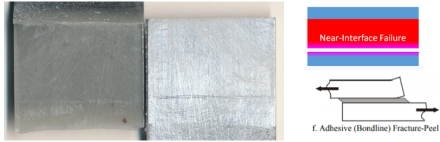
Figure 3.101 Low magnification image after failure for Al-CFRP SLJ bonded with urethane-based adhesive subjected to a strain rate of 15 \text{ s}^{-1} .
