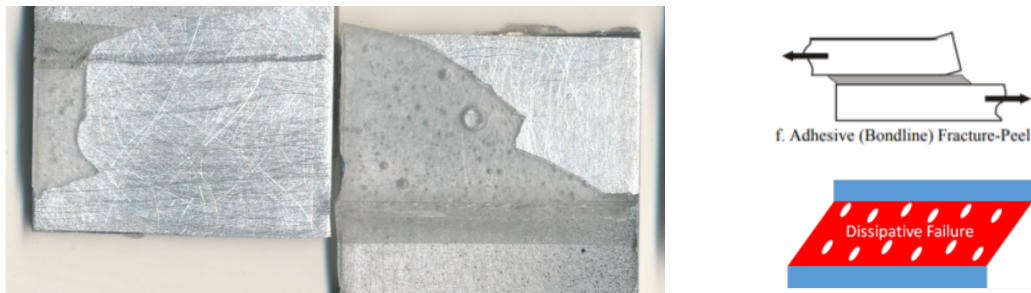
Figure 3.76 Low magnification image after failure for Al-Al SLJ bonded with quick set epoxy tested subjected to a strain rate of 150 \text{ s}^{-1} .
