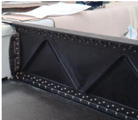
Figure 1.7 Bolted joints in a marine application
