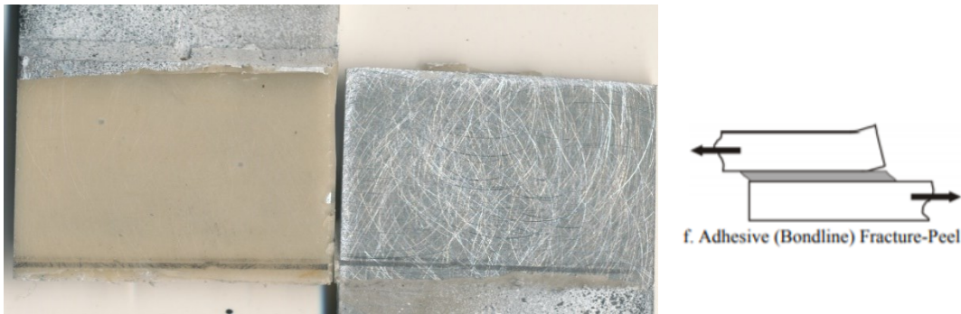
Figure 3.3 Low magnification image after fracture of Al-Al bonded with high strength epoxy under tensile loading conditions at a strain rate of 0.0015 \text{ s}^{-1}
