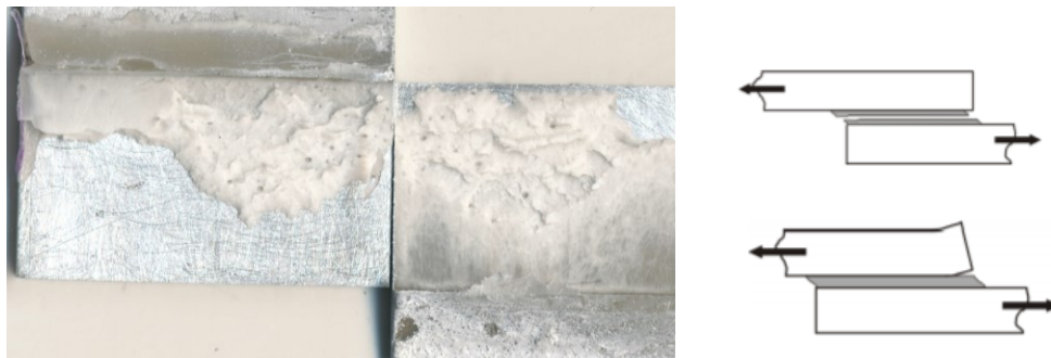
Figure 3.21 Low magnification image after fracture of Al-Al bonded with urethane-based adhesive under tensile loading conditions at a strain rate of 0.15 \text{ s}^{-1}
