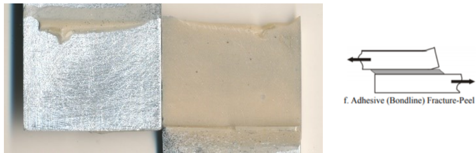
Figure 3.69 Low magnification image after failure for AL-Al SLJ bonded with high strength epoxy subjected to a strain rate of 150 \text{ s}^{-1} .
