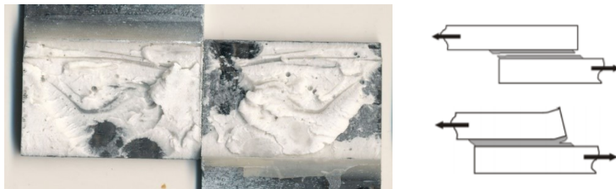
Figure 3.59 Low magnification image after failure for CFRP-CFRP SLJ bonded with urethane-based adhesive subjected to a strain rate of 0.0015 \text{ s}^{-1} .
