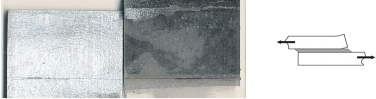
Figure 3.31 Low magnification image after fracture of Al-CFRP bonded with quick set epoxy tested under tensile loading conditions at a strain rate of 0.0015 \text{ s}^{-1} .
