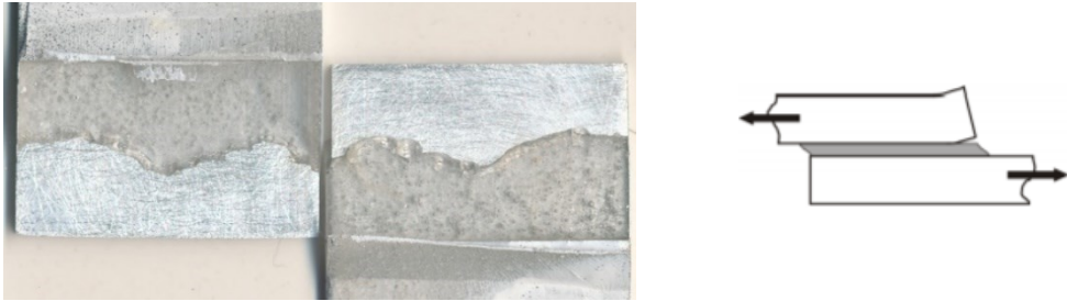
Figure 3.14 Low magnification image after fracture of Al-Al bonded with quick set epoxy under tensile loading conditions at a strain rate of 0.15 \text{ s}^{-1}
