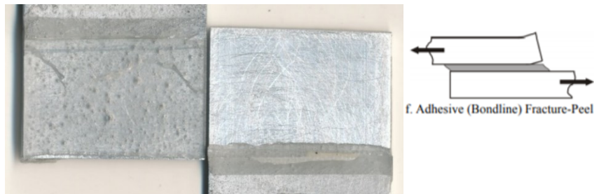
Figure 3.73 Low magnification image after failure for Al-Al SLJ bonded with quick set epoxy subjected to a strain rate of 15 \text{ s}^{-1} .
