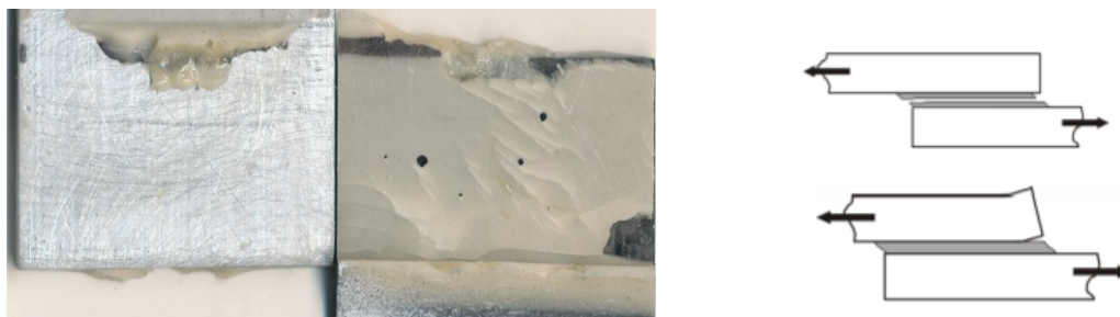
Figure 3.24 Low magnification image after fracture of Al-CFRP SLJ bonded with high strength epoxy at a strain rate of 0.0015 \text{ s}^{-1}
