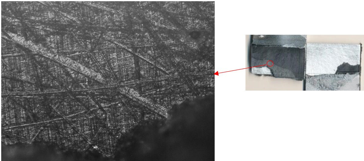
Figure 3.18 Optical microscopy image 10 \times magnification of Al-Al SLJ bonded with urethane-based adhesive tested at a strain rate of 0.0015 \text{ s}^{-1} .
