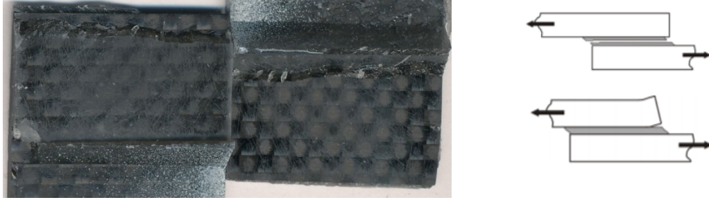
Figure 3.56 Low magnification image after failure for CFRP-CFRP SLJ bonded with quick set epoxy tested at a strain rate of 0.15 \text{ s}^{-1} .
