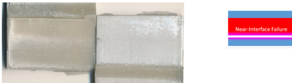
Figure 3.83 Low magnification image after failure for Al-Al SLJ bonded with urethane-based adhesive subjected to a strain rate of 150 \text{ s}^{-1} .
