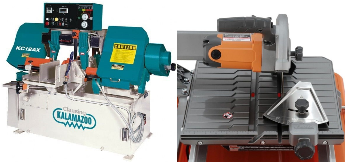
Figure 2.2 (a) Horizontal wet cutting bandsaw (b) Wet tile saw with a diamond coated cutter
