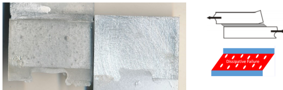
Figure 3.10 Low magnification image after fracture of Al-Al bonded with quick set epoxy at a strain rate of 0.0015 \text{ s}^{-1}
