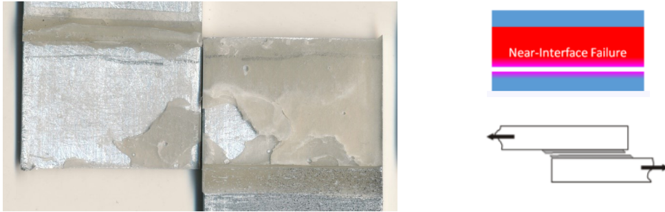
Figure 3.80 Low magnification image after failure for Al-Al SLJ bonded with urethane-based adhesive subjected to a strain rate of 15 \text{ s}^{-1} .
