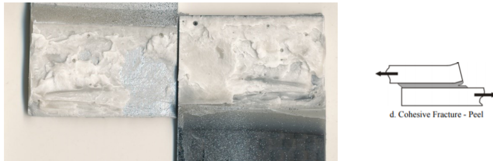
Figure 3.42 Low magnification image for Al-CFRP SLJ bonded with urethane-based adhesive under tensile loading conditions subjected to a strain rate of 0.15 \text{ s}^{-1} .
