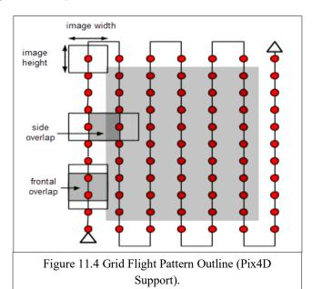
allow for each row to capture imagery in the two adjacent rows. Typically, the overlap is 60% or higher. For densely vegetated areas with complex geometric shapes such as the IRP, overlay is more effective with 85% or higher. If a more sophisticated drone is purchased, a grid pattern can be used to capture imagery of the entire preserve rather than small photo points. See Appendix III-D-1 for more detail.
