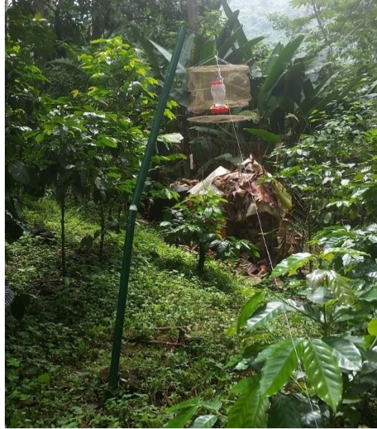
Figure 1. A hummingbird trapping station: standard hummingbird feeder with 25% sucrose solution surrounded by a mesh Hall trap hung from a painted PVC pipe stand. The string shown is a fishing line used to manually open and close the trap.
