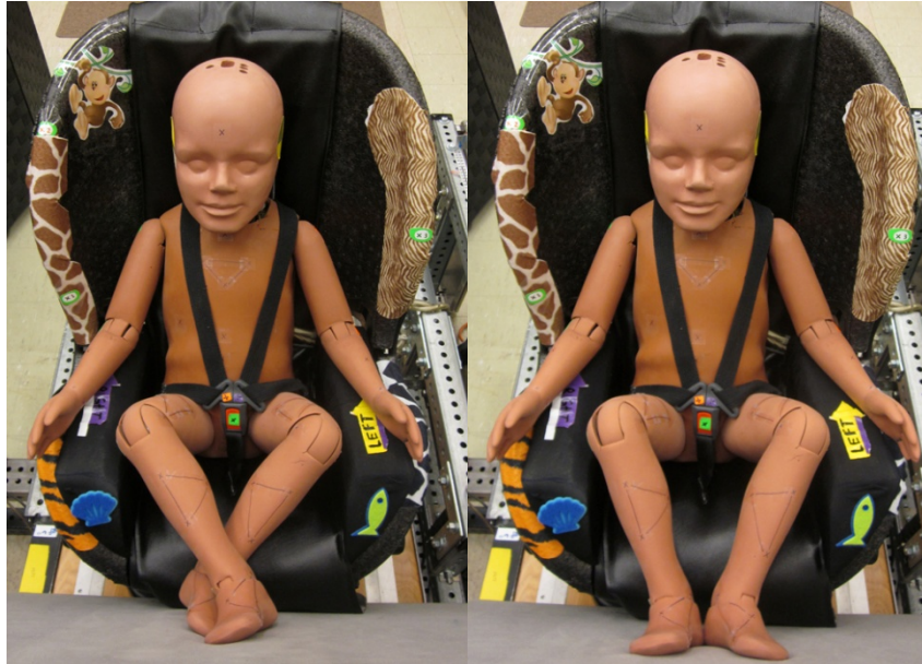
Figure 52. Alternate attempts to place 3YO in crossed leg posture using narrower seat width. Note wrinkling of flesh in the torso due to posterior rotation of the pelvis resulting from force applied at the feet.
