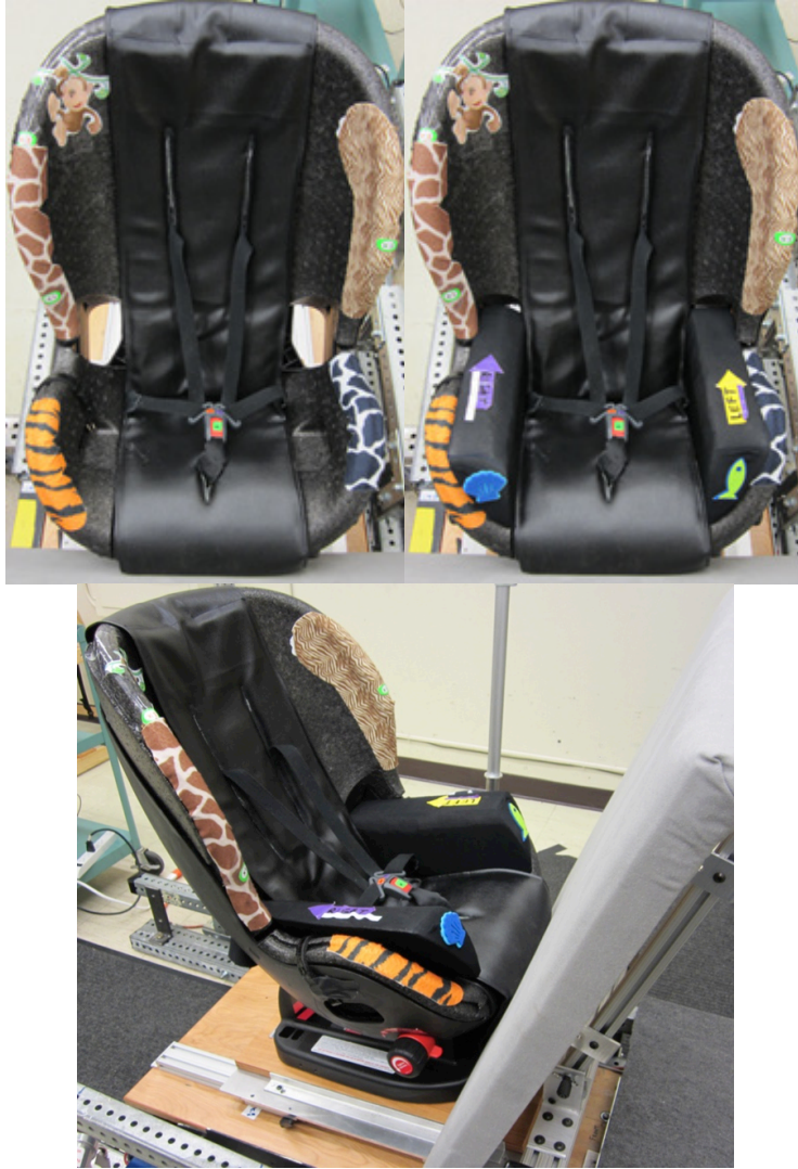
Figure 4. Evenflo Triumph 65L in standard condition (left), with inserts to create a narrower seat width (right), and mounted to test fixture (below).
