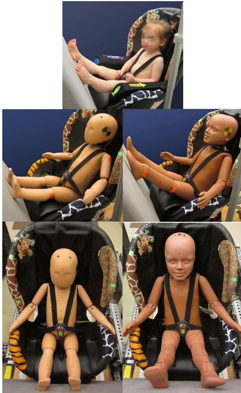
Figure 49. Legs elevated position for volunteer child (top), 18MO ATD (left), and 3YO ATD (right).
