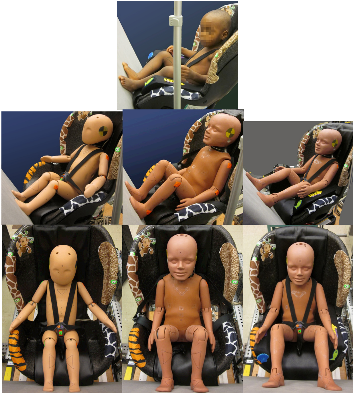
Figure 45. Legs relaxed position for a child volunteer (top), the 18MO ATD (left), 3YO ATD relaxed (middle), and 3YO ATD relaxed with feet apart (right)
