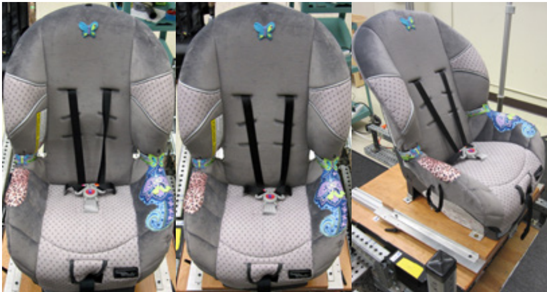
Figure 5. Graco ComfortSport convertible attached to the mounting board (upper left), foam insert used to simulate shorter cushion length (upper right), in standard condition (lower left), in shorter seat cushion (lower mid), and installed on test fixture (lower right.)
