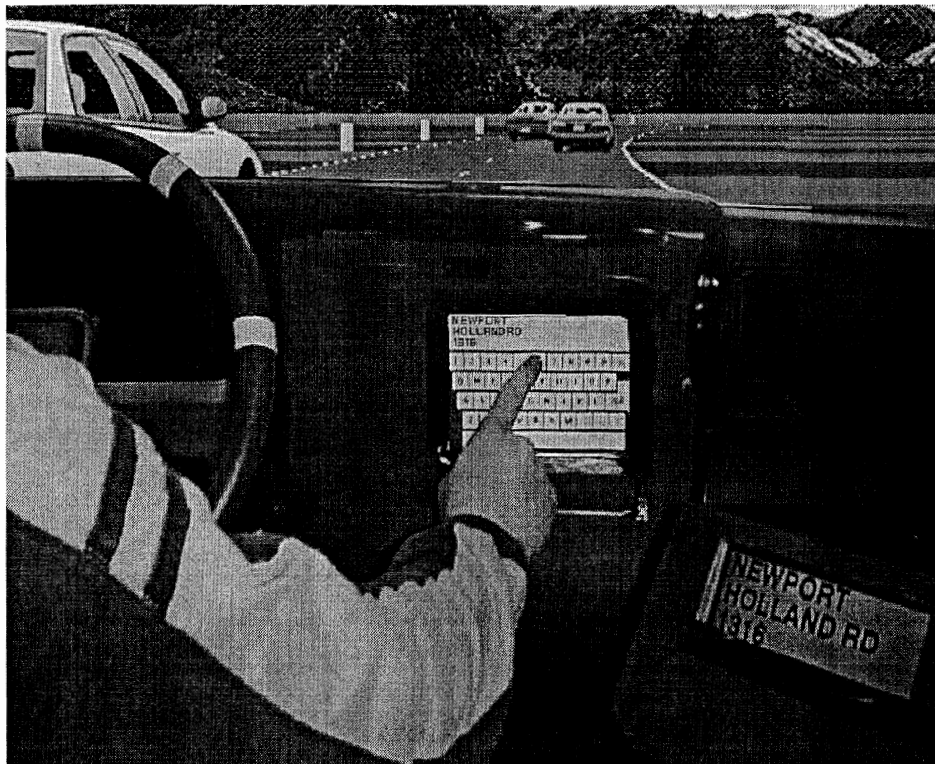
Figure 6. Driver's view of the road and touch screen (Note: The touch-screen keyboard and road scene were enhanced in this image for clarity)
