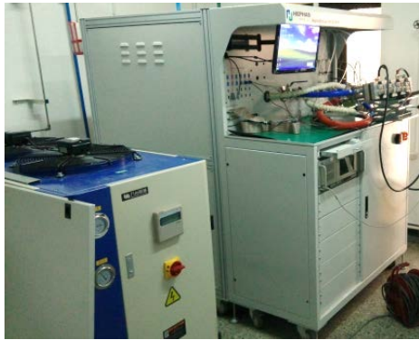
(a) 10kw fuel cell test bench
