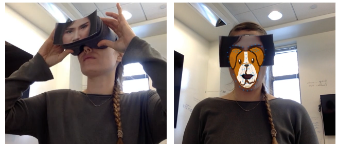
Figure 8: Use camera-based face tracking while in VR through taping a photo of a half face onto a VR headset.
