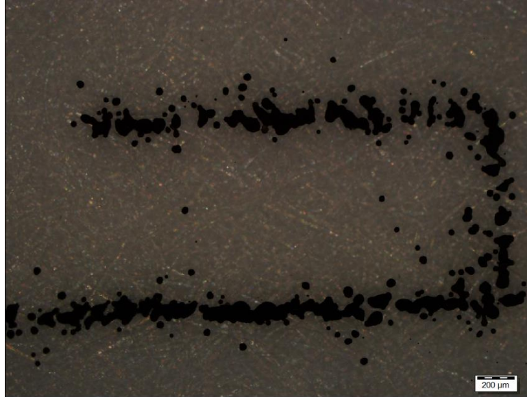
Figure 6-1: Sumi-ink on premium paper, at 157^\circ\text{C} , a resolution of 90\mu\text{m} is reached
