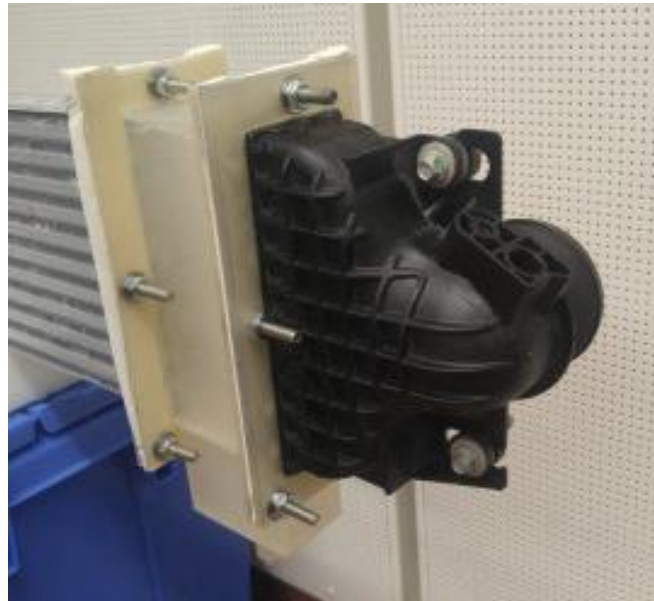
Figure 3-30. A prototype of separator integrated in charge air cooler
