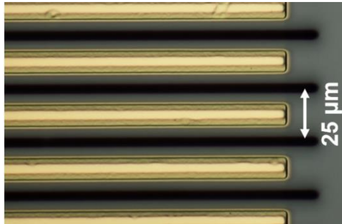
Figure 8-11: Au deposited between SiO 2 pillars with shadow mask. Thinner Au exists on the top and bottom of the drawn feature due to the angle of deposition and the 25 μm offset of the shadow mask from the wafer surface.
