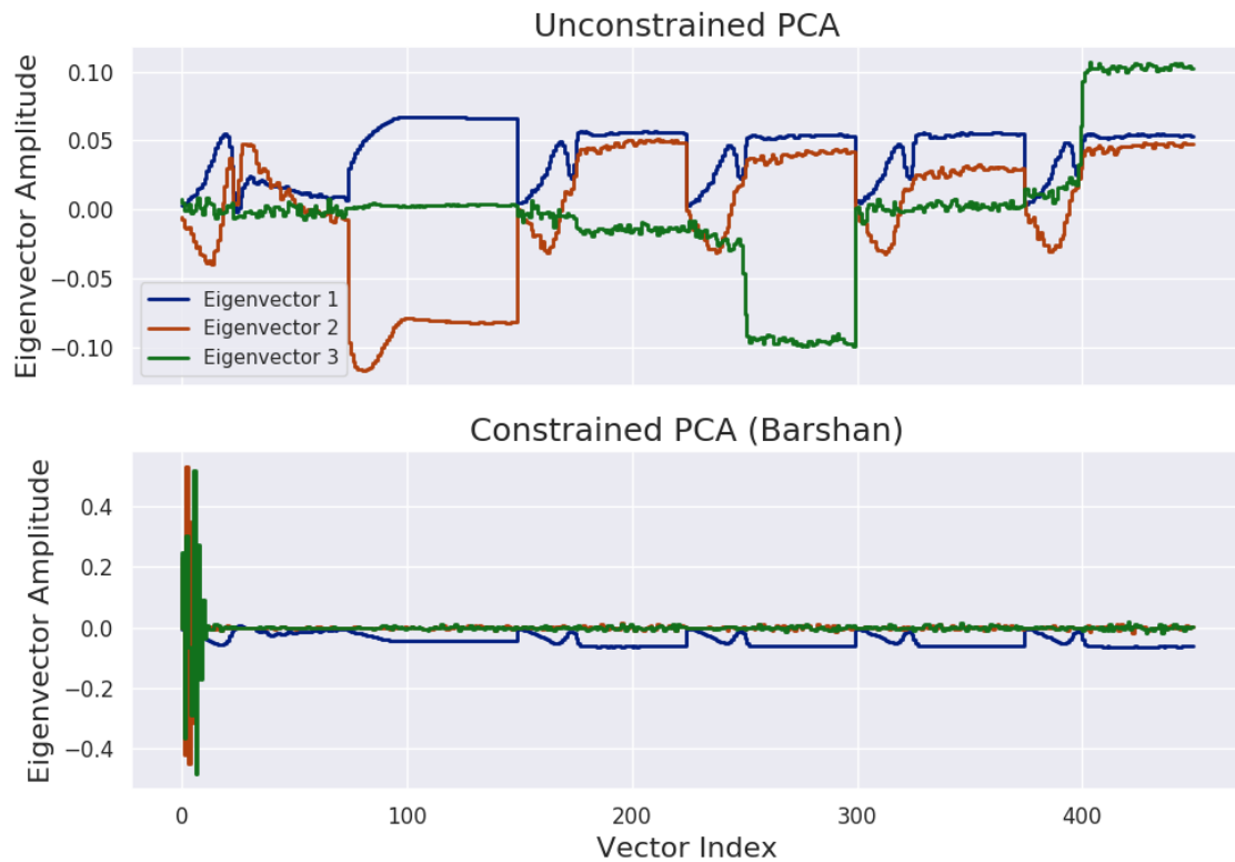
Figure 4.21: Eigenvectors for the first three principal components obtained by unconstrained PCA (top) and Barshan's method (bottom).
