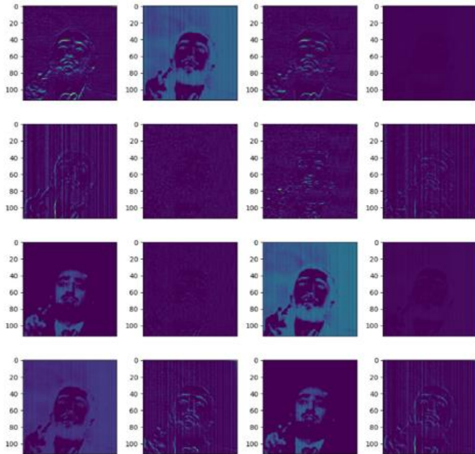
(c) The first layer output (shown only 16 out of 64 channels) from test image with SqueezeDet
