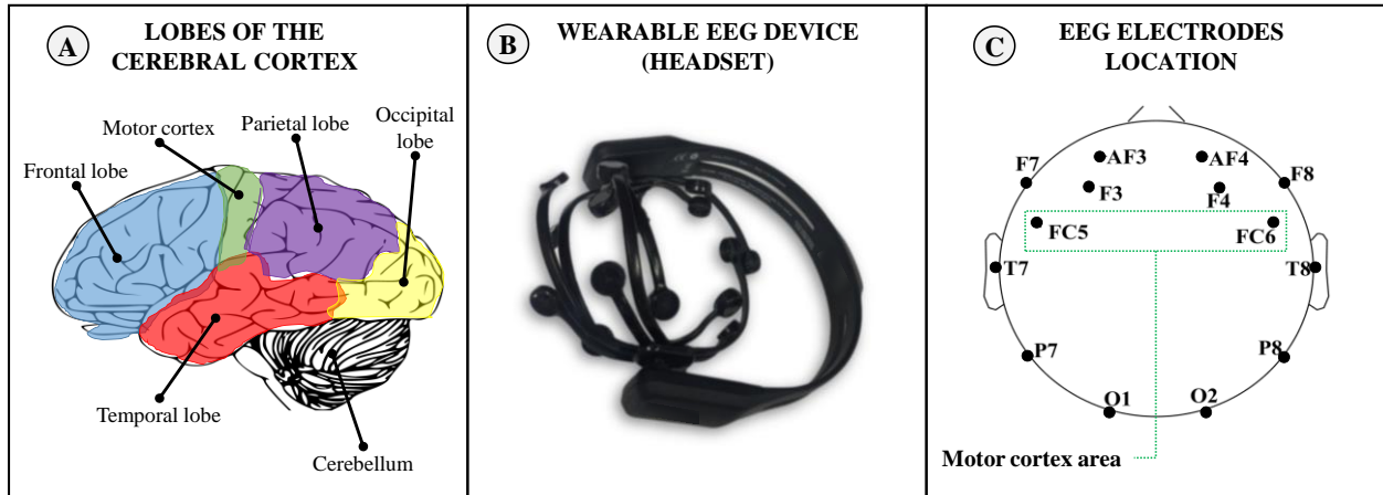
Figure 2.1. An overview of wearable EEG: (a) the cerebral cortex of the brain; (b) an example of the wearable EEG device; and (c) EEG electrode placements.
