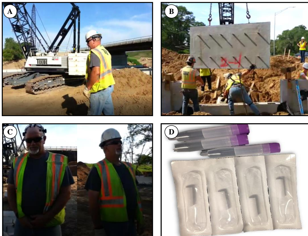
Figure A.4 EEG data collection in field: (a) Low stress experimental tasks (e.g., working on the ground level and working right after break); (b) High stress experimental tasks (e.g., working at top of a ladder, working in a confined space, and working in dangerous environment); (c) Wearable EEG headset fit into worker's safety hardhat; (d) Salivary cortisol samples kit.
