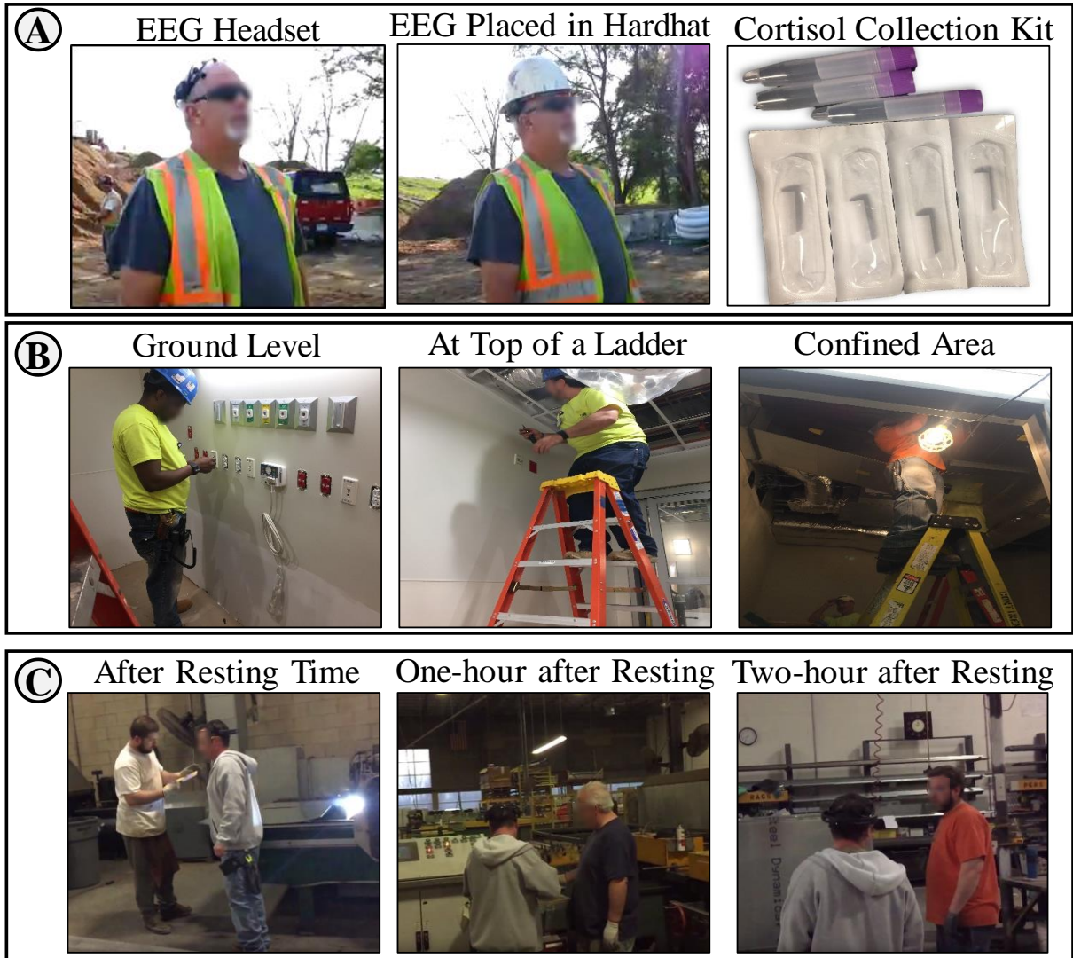
Figure 5.3 Construction workers’ dataset data collection: (a) Wearable EEG headset, location of electrodes, and salivary cortisol sample collection kit; (b) Working in the work area with different hazard levels; (c) working with different level of tiredness.
