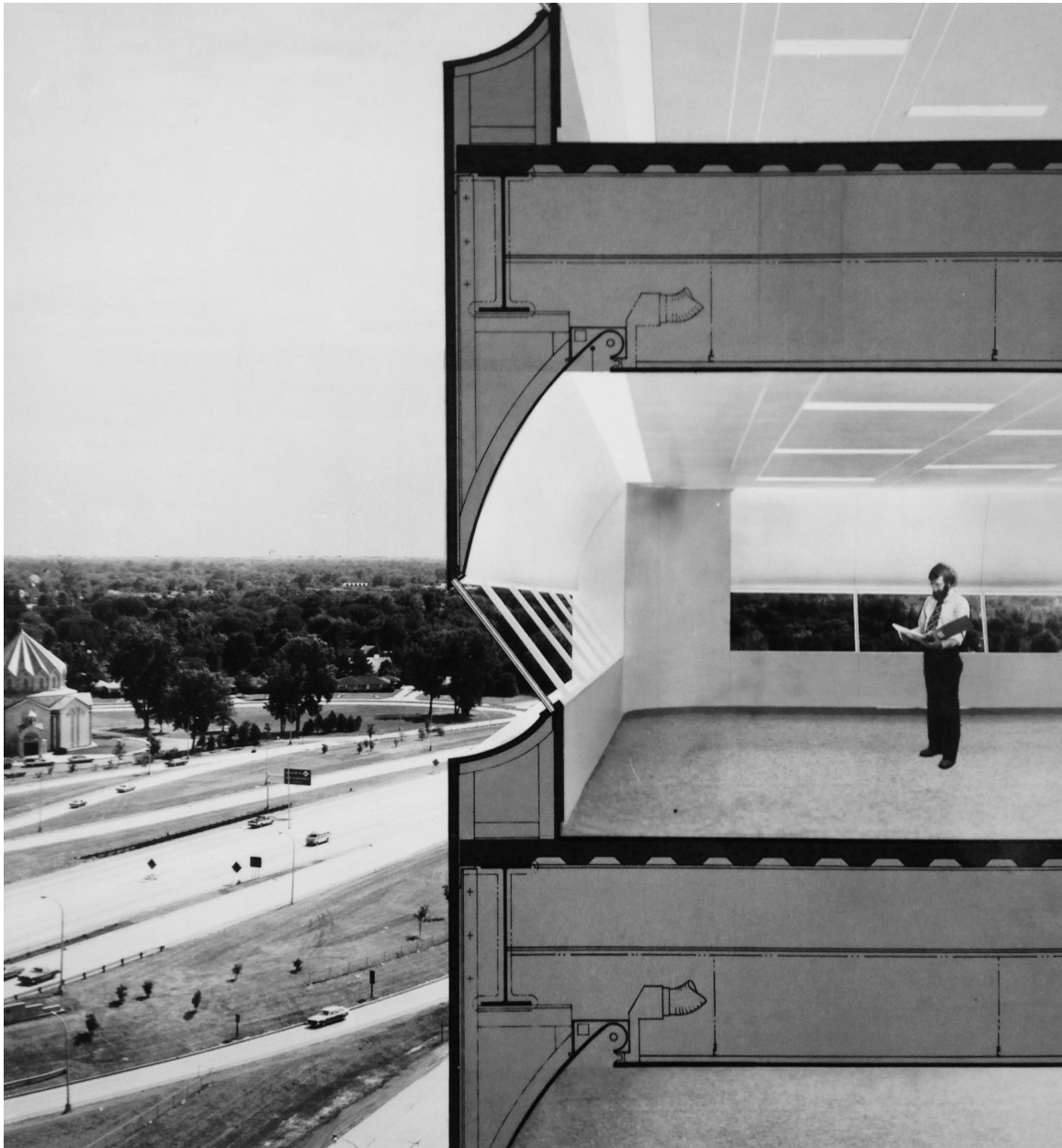
Figure 4.49 GBA, photomontage of IBM Regional Office, Southfield, Michigan showing concave reflectors and canted windows. Box 13, GBP, BHL.
