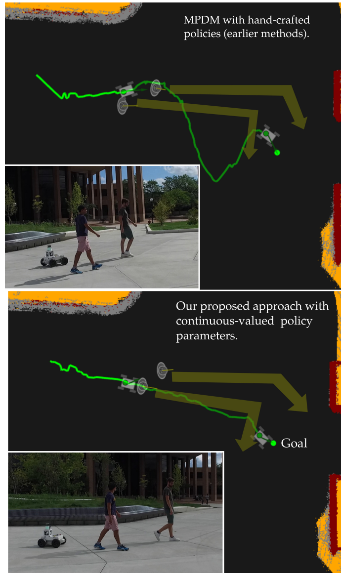
Figure 5.7: Robot trajectories from a real-world experiment. Two agents walk closely in front of the robot as it navigates towards its goal. The agents arbitrarily change speed and suddenly turn acutely near the robot’s goal (star). The arrows mark the general trajectory of the pedestrians. Salient locations are marked by circles. The undesirable behavior from MPDM with hand-crafted policies ( \Pi_{hc} ) stems from switching between very distinct policies ( Left ). At location 1, the MPDM chooses to overtake the agents at a High speed towards the Left of the goal (see Sec. 5.4.1). However, the pedestrians also speed up slightly and the robot still lags behind as it approaches location 2 at which point, in order to make more Progress , the robot switches strategies and attempts to overtake from the other side (towards the Right of the goal). As the robot approaches location 3, the agents start turning acutely. and in order to reduce Blame , rather than going straight towards the goal, the robot tries to swerve around the agent from the Left of its goal. This extreme switch causes the robot to deviate once again. By allowing smoother transitions in nominal speed and heading, C-MPDM avoids unnecessary deviation ( Right ).
