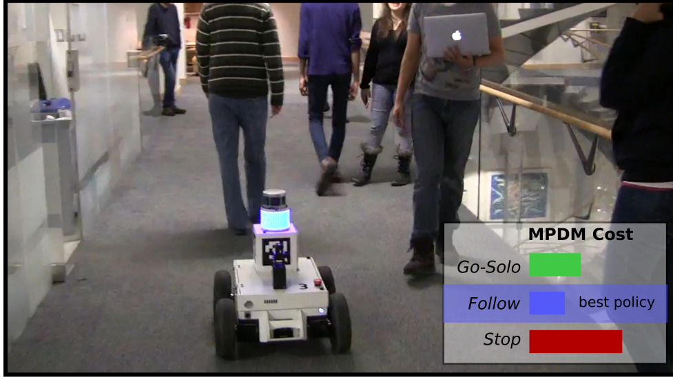
Figure 3.1: Navigating a hallway by switching between different policies. Our approach implemented and tested using the MAGIC [148] robot platform. We show that our algorithm is able to navigate successfully on an indoor environment amongst people. MPDM allows the robot to choose between policies. In this case, the robot decides to Follow the person in front rather than try to overtake him.
