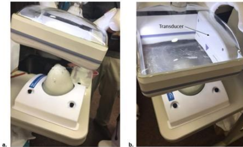
Figure 5.3: ABUS image acquisition setup on uncompressed phantom
