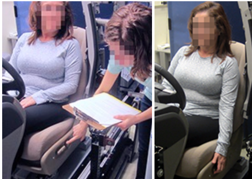
Figure 17. Investigator reading script and demonstrating controls for adjustable components on the vehicle mockup (left) and participant adjusting the seat before donning the belt (right)
