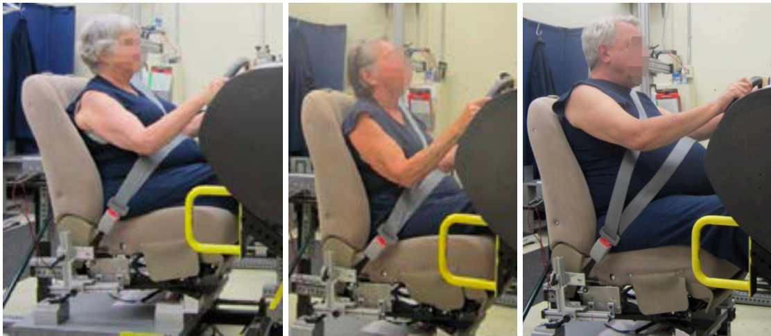
Figure 1. Examples of poor belt fit on participants in Reed et al 2013.
