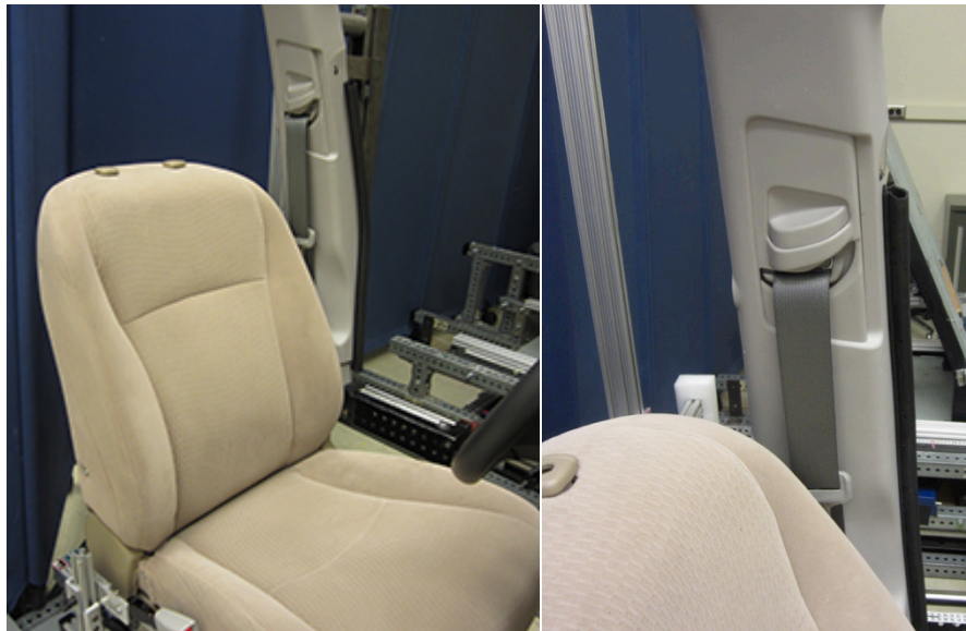
Figure 14. Vehicle mockup detail of seat and upper anchorage with D-ring adjusted to one stop below bottom and its pivot center mounted 21° from vertical with respect to the seat H-point (J826)
