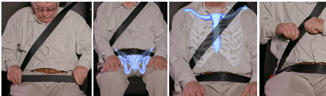
Figure 2. Still images from video intervention demonstrating moving the lap belt low across the hips, centered on collarbone and snug against the body
