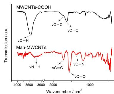
Figure 2. Infrared spectra of MWCNTs-COOH and Man-MWCNTs.
