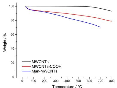
**Figure 3.** Thermogravimetric profiles of MWCNTs, MWCNTs-COOH and Man-MWCNTs.
