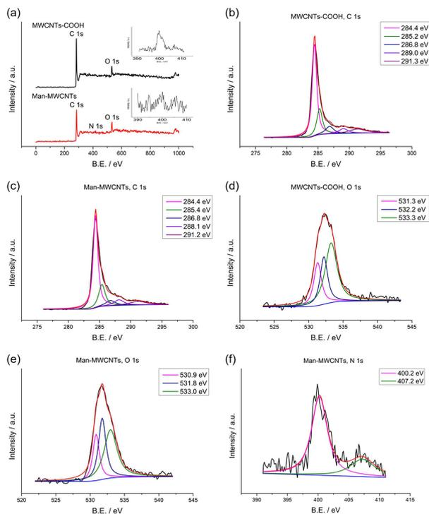
**Figure 4.** Results of XPS analysis of the MWCNTs-COOH and Man-MWCNTs: (a) XPS survey scan spectra of MWCNTs-COOH and Man-MWCNTs. The inset is magnification of the N1s region in MWCNTs-COOH and Man-MWCNTs spectrum. (b,c) High resolution fitted XPS C1s spectra of MWCNTs-COOH and Man-MWCNTs. (d,e) High resolution fitted XPS O1s spectra of MWCNTs-COOH and Man-MWCNTs. (f) High resolution fitted XPS N1s spectra of Man-MWCNTs.
