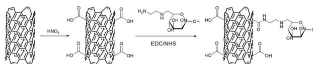
Figure 1. Synthesis of Man-MWCNTs.
