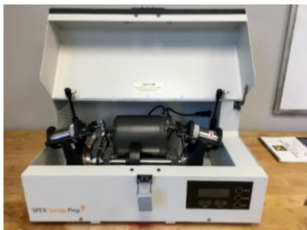
Figure 36 SPEX SamplePrep 8000 dual high energy ball mill
