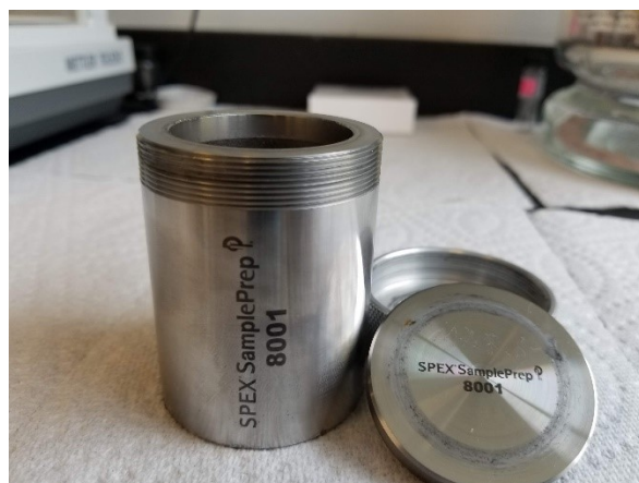
Figure 37 SPEX 8001 hardened steel vial used for the milling
