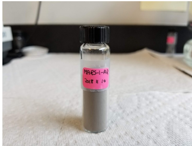
Figure 35 The as-received, pre-alloyed gas-atomized maraging steel powder
