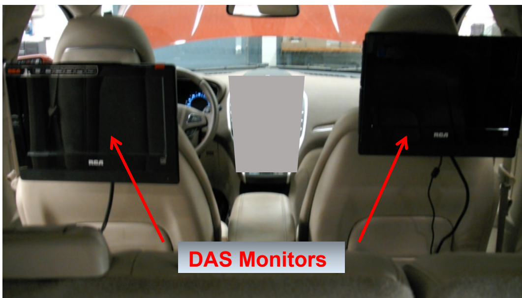
Figure 5: DAS Monitors for Test Identification and Monitoring
