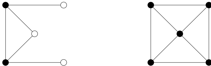
Figure 5.2: Left to right: a network N with boundary nodes marked in white and the associated graph \widehat{\Gamma} = W_5 .
