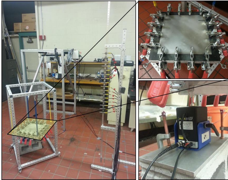
Figure 5.13: Experimental test apparatus for the remote acoustic measurement of vibrating plates. The nominally clamped test plate (top right) is excited from below with an electrodynamic shaker (bottom right). An array of microphones (left) placed roughly 1 m from the plates were used to record radiated sound.
