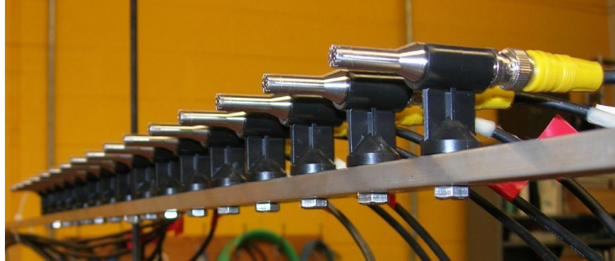
Figure 2.9: Linear array of 16 PCB 130E20 electret microphones used in this thesis. This horizontal configuration with 2-inch spacing was one of a multiple of array configurations available.
