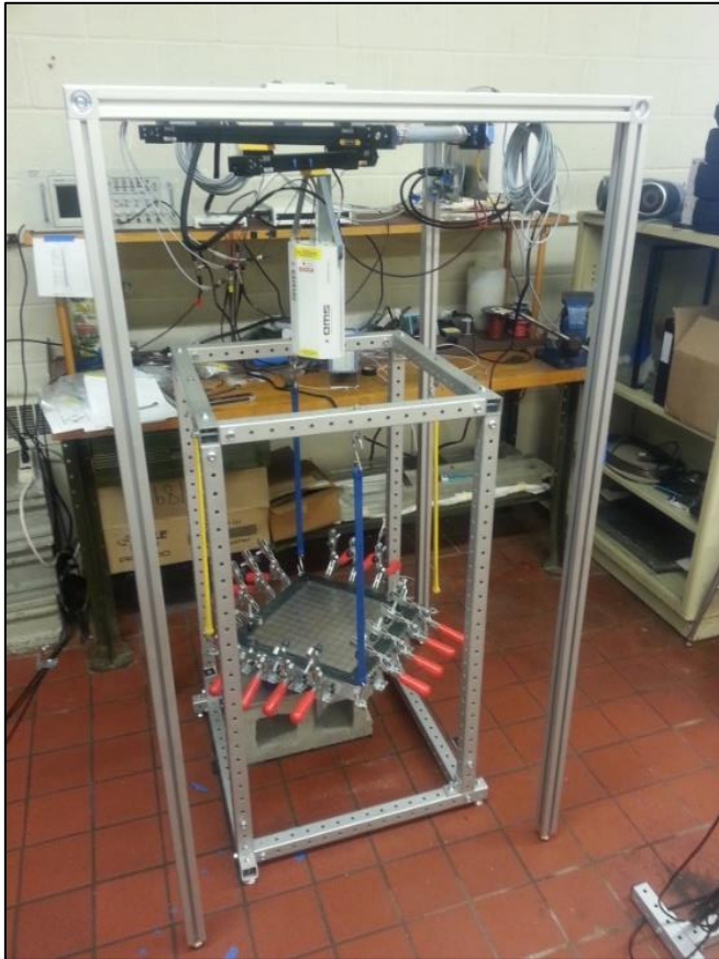
Figure 2.15: Laser Doppler vibrometer setup. The single point OMS LP-01 LDV is mounted to a two-axis automated gantry with 46 x 46 cm area of motion, allowing for full surface scans of the test plate apparatus.
