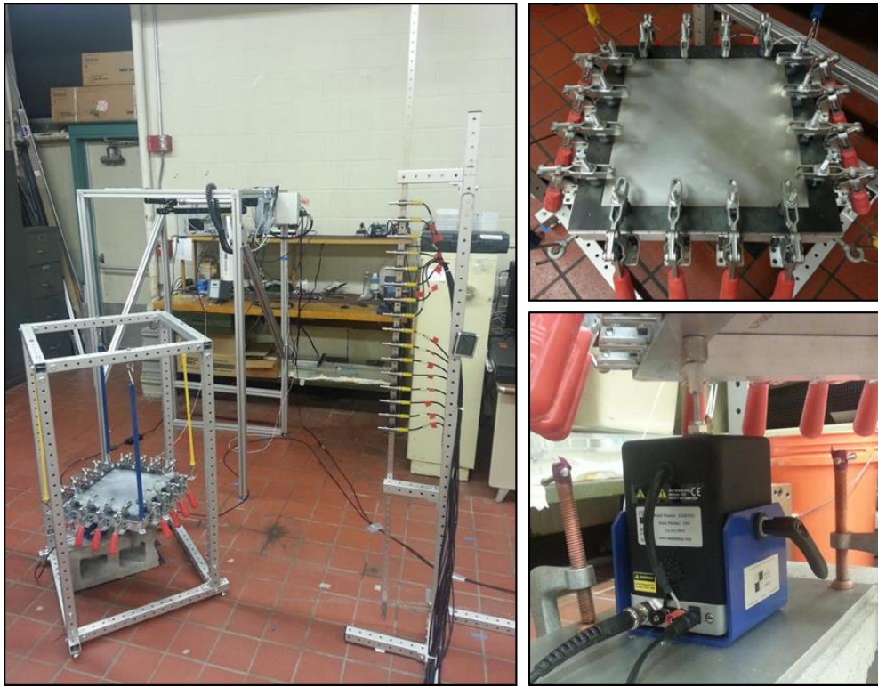
Figure 3.2: Experimental setup with plate apparatus and 15 receiver vertical array at 1m range in the test environment (left), detailed view of clamped plate system (top right), and 7 lbf shaker providing base excitation of the plate (bottom right).
