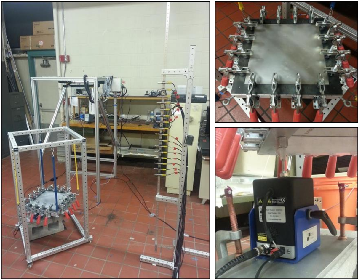
Figure 2.13: The plate vibration rig and microphone array (left). A close-up of a mounted 1/16'' aluminum plate is shown (top right). An electrodynamic shaker (bottom right) drives the system from the rigid base, thereby base-exciting the test plate. A force couple, in-line with the shaker, allows for simultaneous measurement of excitation forcing into the system.
