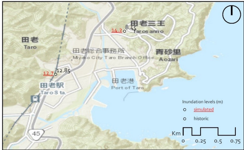
Figure A.15: Comparison of simulated vs observed water inundation as validation for the 1896 tsunami.
