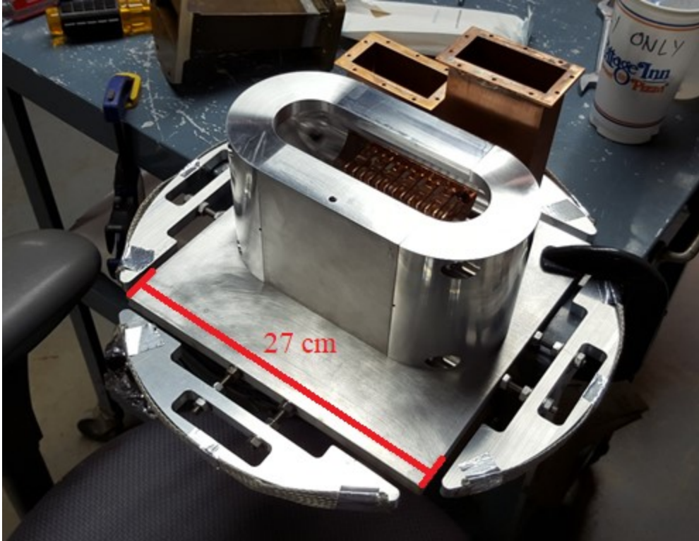
Figure 3.13: Inner housing mounted to the inner wheel. The steel braid fastened to the wheel ensures good electrical contact with the vacuum chamber.
