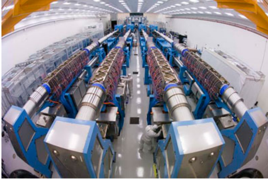
Figure 1.5 A picture of the experimental bay at Omega-EP. The optics associated with each of the four beamlines are seen in the foreground, the vacuum chamber is at the far end of the room.
