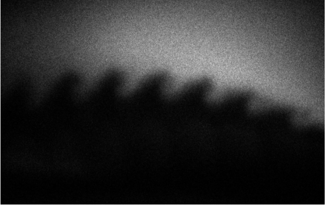
Figure 4.7 A radiograph of a post-shock staircase perturbation. The initial height of the stair was 25 \mu\text{m} , and the width is 100 \mu\text{m} . The image was taken 24 ns after the drive beams are first incident on the ablator. The leftmost visible spike is \sim 14 ns post-shock, and each stair is shocked 0.625 ns after the vortex to its left while the shock remains planar.
