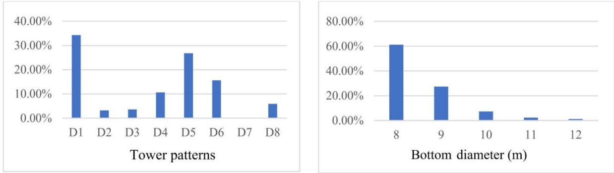
Figure 74: The clustered column charts illustrate the percentage of the lightweight generated solutions based on the tower patterns and bottom diameter.
