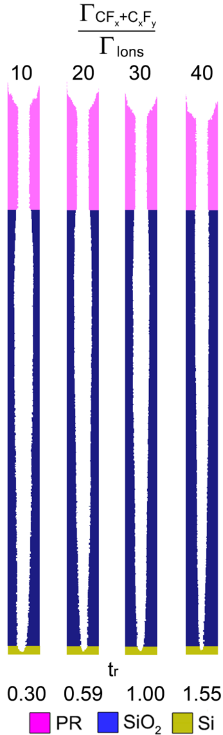
Fig. 6.13 Final etch profiles (central slice) with 10% over-etch of during HAR etching for different (CF_x + C_xF_y)/ion flux ratios from 5 to 40. Only photoresist (PR), SiO_2 and Si are shown with the complex and polymers being blanked out. The (CF_x + C_xF_y)/ion flux ratio in the base case is 30. The fluxes of ions were varied while the fluxes of CF_x and C_xF_y remained constant. The same IEADs from the base case were used in all cases. The relative etch time, t_r , is listed below each feature.
