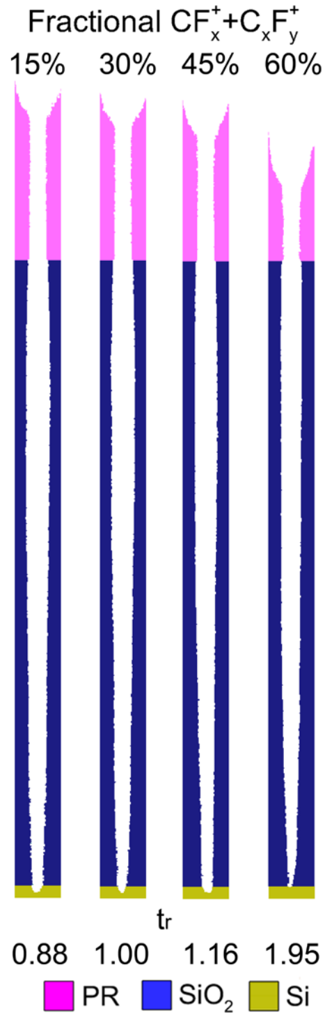
Fig. 6.15 Final etching profiles (central slice) with 10% over-etch for HAR etching for different fractional CF_x^+ and C_xF_y^+ . Only the photoresist (PR), SiO_2 and Si are shown with the complex and polymers being blanked out. The fractional CF_x^+ and C_xF_y^+ in the base case is 15%. The fluxes of CF_x^+ and C_xF_y^+ ions were varied while the total ion flux was maintained constant by decreasing adjusting the flux of Ar^+ . The same IEADs from the base case were used for all cases. The relative etch time, t_r , is listed below each feature.
