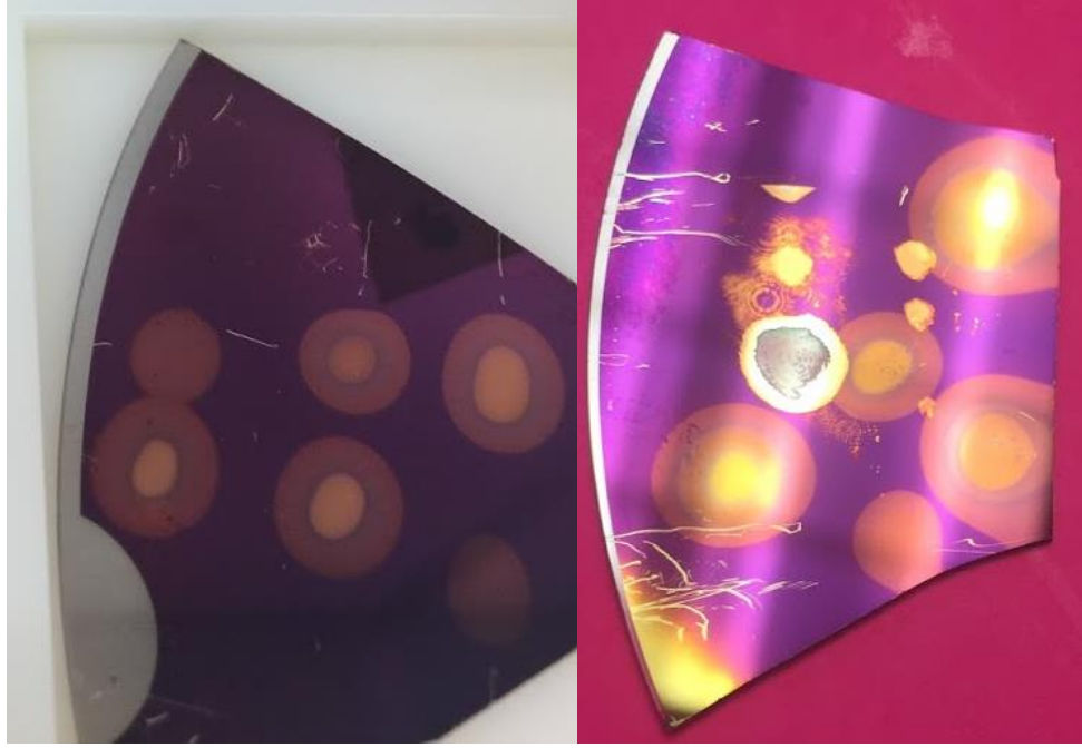
Figure 52. The laser annealing method to produce different color gradient in the stack that consists of GeTe, SiO 2 and TiO 2 films (left). Film evaporation due to excessive heat for a sample without the protecting oxide layer (right).
