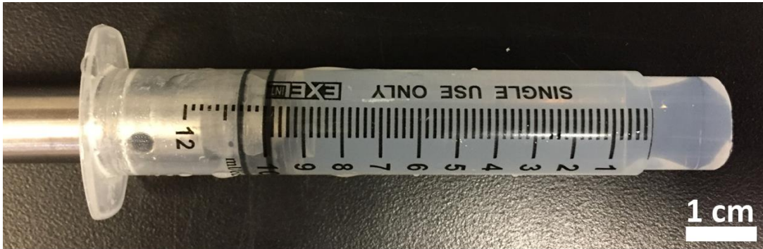
Figure 4. 1. Photograph of agarose gel phantom in modified syringe used for molding and fixturing the gel during experimentation.
