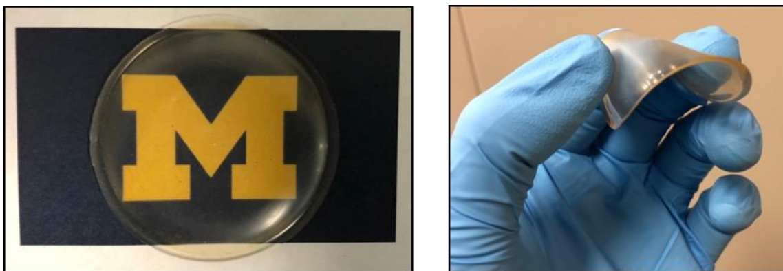
Figure 5.5 Recycled 1 Ph : 1 Me silicone resin after recycling and in situ modification to left) 1 Ph : 4 Me has right) increased flexibility
