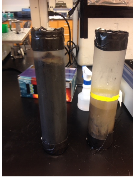
Figure C3. Image of a sediment core taken from the Middle Island Sinkhole (left) and a core taken from Lake Huron (right). The difference in color between the two cores can be attributed to a difference in organic matter burial, with organic C contents for MIS >2x that of LH (Nold et al., 2013; Kinsman-Costello et al., 2017; Rico & Sheldon, 2019).
