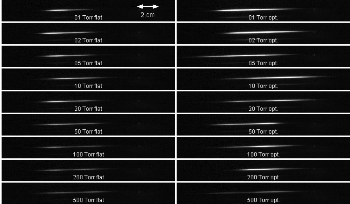
Figure 6.10: Comparison of images of the filament plasma fluorescence when the mirror is flat (left column) versus optimized with the antenna at \theta = 25^\circ (right column). The direction of laser propagation is right to left.
