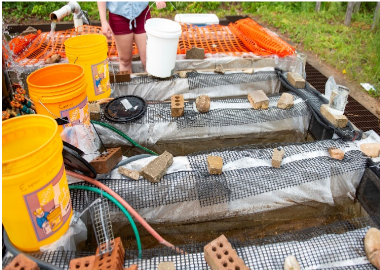
Figure 1: University of Michigan Stream Research Facility stream lab set up for Trial 1. Drip buckets shown alongside left of the picture and hoses connected to buckets flowing water into artificial stream.
