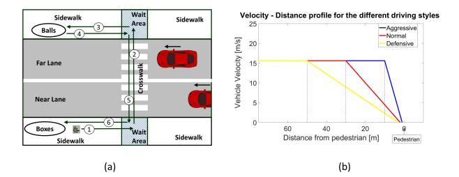
**Figure 3.** (a) Pedestrian state divisions in the virtual environment. Numbered arrows indicate a typical pedestrian path while doing the task. (b) Driving profiles for the three driving behaviors when the pedestrian is on the road in the same lane as the AV. To achieve the specified stopping distance and slow speeds, defensive behavior decelerated much earlier than normal or aggressive.
