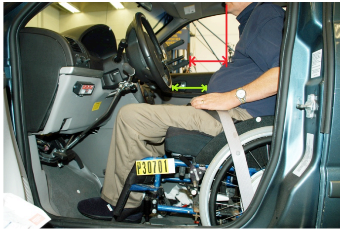
Figure __: Driver's Chin and Abdomen Position Relative to the Steering Grip Enhancer and the Lower Rim of the Steering Wheel.
