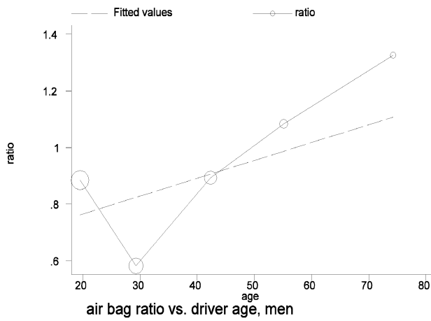
Figure 2.2.4-19 Ratio of driver fatality risks in cars with and without air bags, versus driver age, male drivers. Single car crashes, left side impact.
