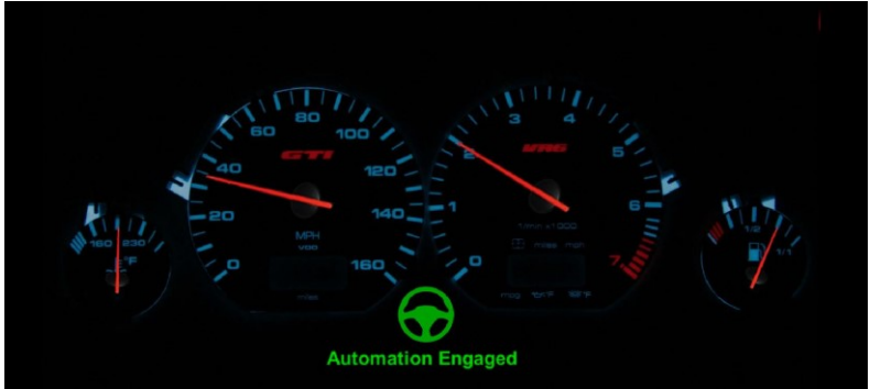
Figure 2-7 Showing the icon when the CAD system is activated or turned ON or engaged
