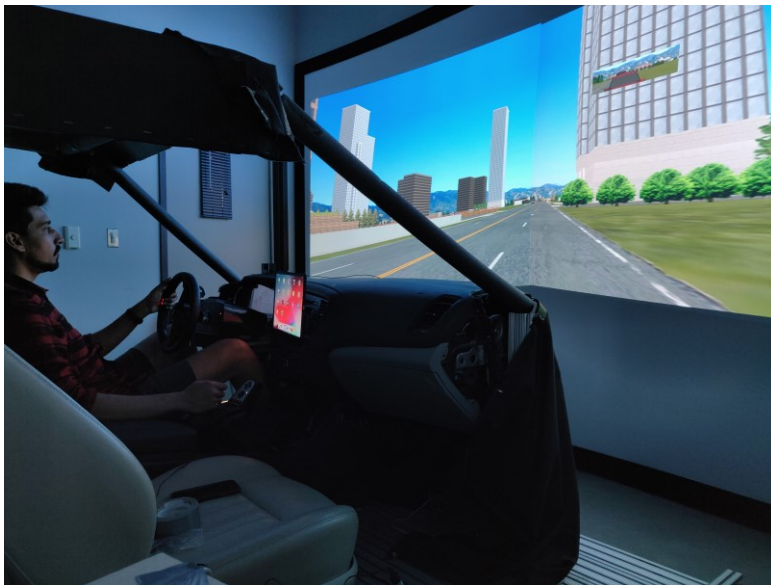
Figure 2-2 Car Buck depicting Gear Shifter, Infotainment Screen and Driving Scenario
