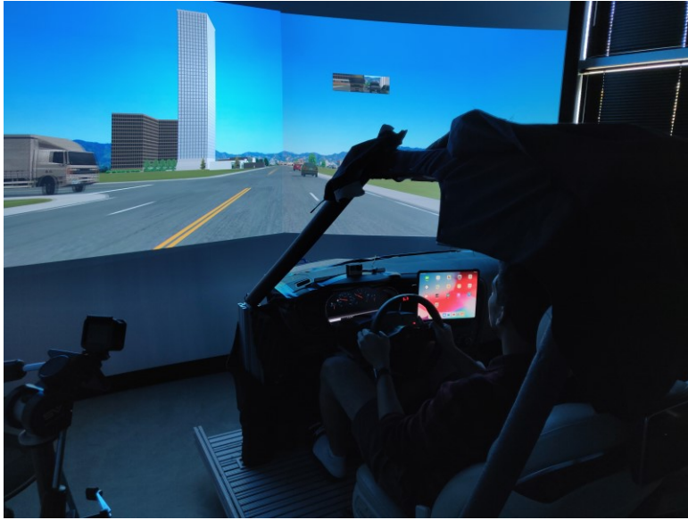
Figure 2-1 Driving Simulator Lab depicting GoPro device, Instrument Cluster of CAD system, Infotainment Screen and Driving Scenario on the Projector Screen
