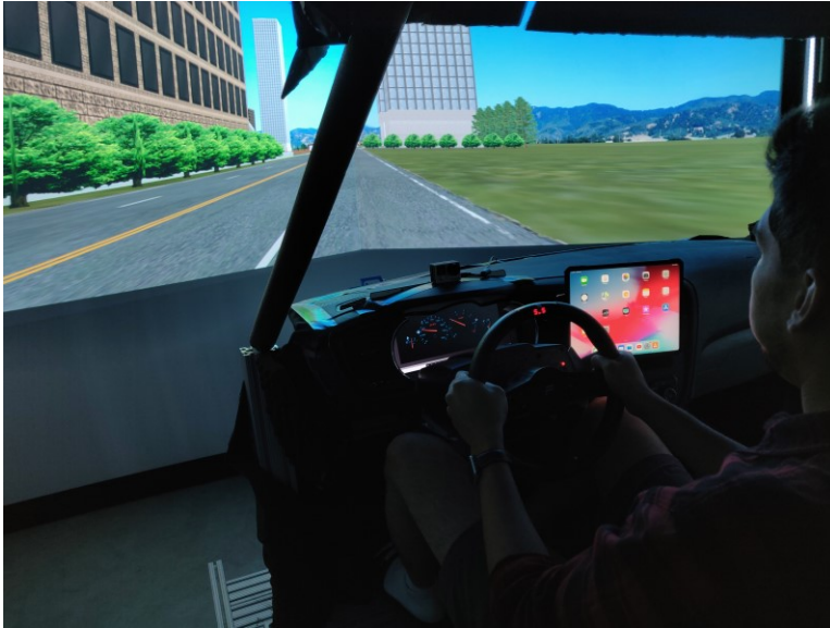
Figure 2-3 A zoomed-in view of the Car Buck to depict Paddle Shifters in between Steering wheel and Instrument Cluster for activating CAD System
