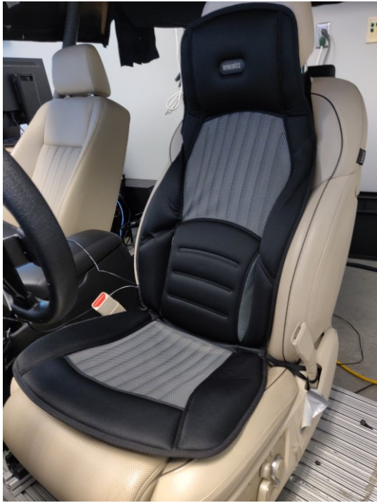
Figure 2-8 Vibrotactile Mode of the Multimodal TOR
